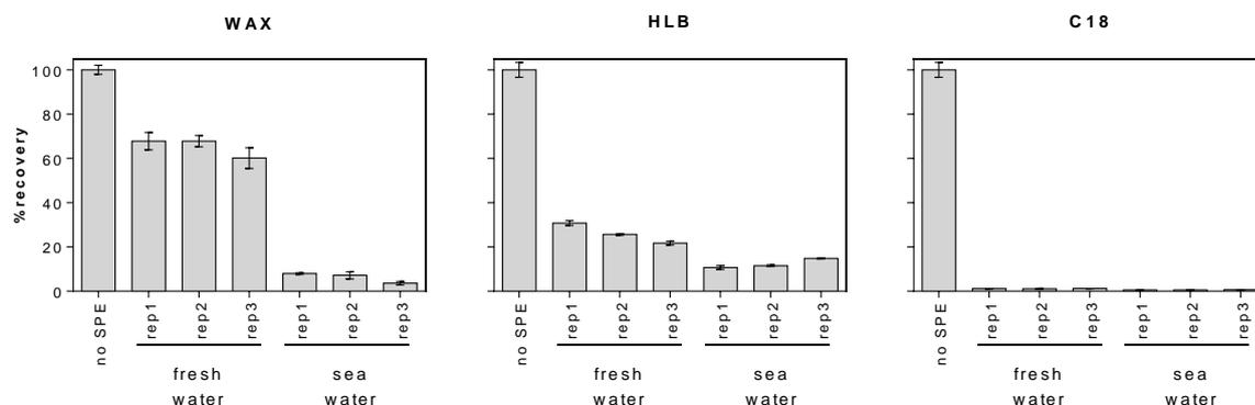
**Figure 5:** SPE recoveries. Error bars represent  $\pm$  one standard deviation of three technical replicates.
