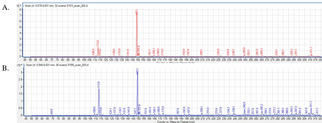
**Figure 8:** Mass spectrum of aqueous SIBX after 10 min (B.) shows no detectable degradation products compared to t = 0 (A.). Note that the peak at m/z 113 corresponds to a common background ion from trifluoroacetic acid.
