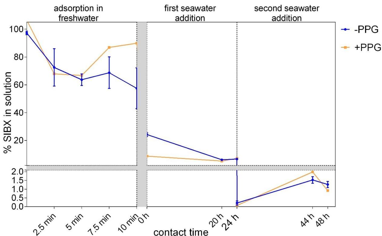
**Figure 7:** Results from the partitioning study. Error bars represent  $\pm$  one standard deviation of three experimental replicates.
