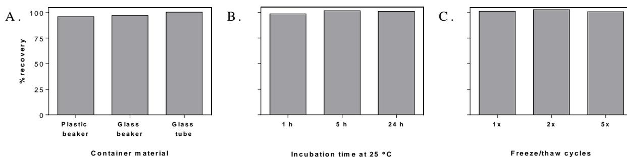
**Figure 6:** SIBX stability. (A) Stability of a 1  $\mu\text{g/ml}$  solution of SIBX in distilled water over 24 h in different containers. (B) Stability over time of a 1  $\mu\text{g/ml}$  solution of SIBX in distilled water. (C) Stability of SIBX after several freeze/thaw cycles.
